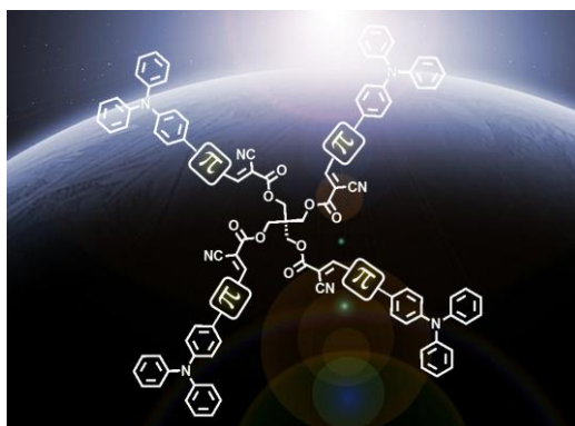
Figure 1 – Illustration of a triphenylamine based tetramer used as molecular donor in BHJ solar cells
