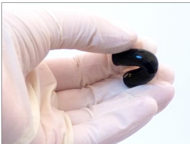
Figure 1 – Polyaniline cryogel: soft, flexible, conducting
